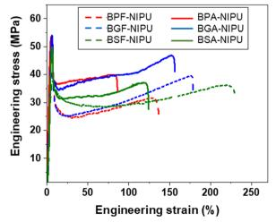
Fig. 2 Representative tensile engineering stress vs. engineering strain curves for NIPUs acquired from uniaxial tensile testing using a load cell of 100 N and a strain rate of 10% min $^{-1}$  at  $\sim$ 20 °C.
