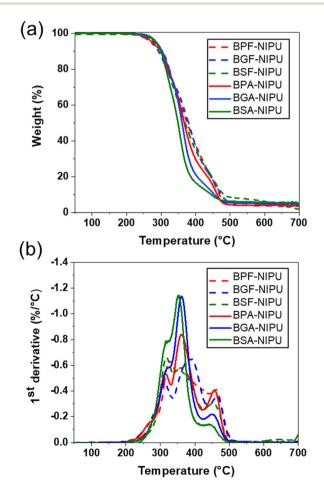
Fig. 4 (a) TGA thermograms of NIPUs in N<sub>2</sub> atmosphere; sample weight (%) as a function of temperature with a heating rate of 10 °C min<sup>-1</sup>, and (b) the first derivative of the weight remaining (%/°C) as a function of temperature for all NIPUs
