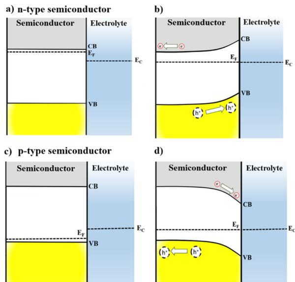
Fig. 1 Energy diagrams for n-type and p-type semiconductor electrodes immersed in an electrolyte with electrochemical potential ( $E_{EC}$ ) at non-equilibrium (a) and (c) and in equilibrium (b) and (d) with the Fermi level of the semiconductor ( $E_F$ ).
