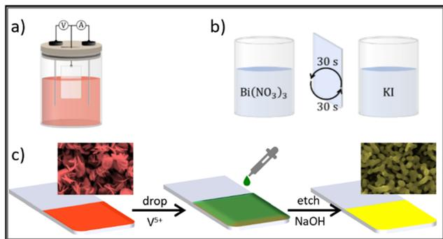
Fig. 12 BiVO<sub>4</sub> synthesis via BiOI template through: (a) electrodeposition; (b) SILAR; and (c) drop cast of V precursor for thermal conversion BiOI → BiVO<sub>4</sub> common to both approaches.
