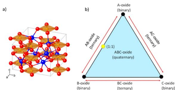
**Fig. 14** (a) The CuBi<sub>2</sub>O<sub>4</sub> crystal structure as viewed at an arbitrary angle. The Bi, Cu, and O atoms are represented by blue, orange, and red spheres, respectively. Reprinted (adapted) with permission from ref. 16 Copyright 2016 American Chemical Society. (b) Graphical visualization of ternary and quaternary oxides, for generic cases. Adapted from ref. 155 according to (CC BY, <https://creativecommons.org/licenses/by/4.0/>) ©The Author(s) 2018. Published by ECS.
