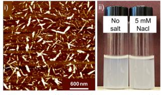
Fig. 7 AFM images of (a) HCl(aq)-CNCs after exposure to H2SO4(aq) (control) and (c) after a 1:1 CNC-to-oligosaccharide surface modification. Also shown are photographs to demonstrate the colloidal stability of 0.1 wt% (b) HCl(ag)-CNCs after exposure to H<sub>2</sub>SO<sub>4</sub>(ag) and (d) HCl(ag)-CNCs + Oligo (1:1) after 24 h without salt and with 5 mM NaCl.
