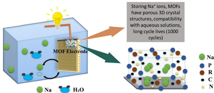
Fig. 8 The application of MOFs in sodium ion batteries.<sup>130</sup>
