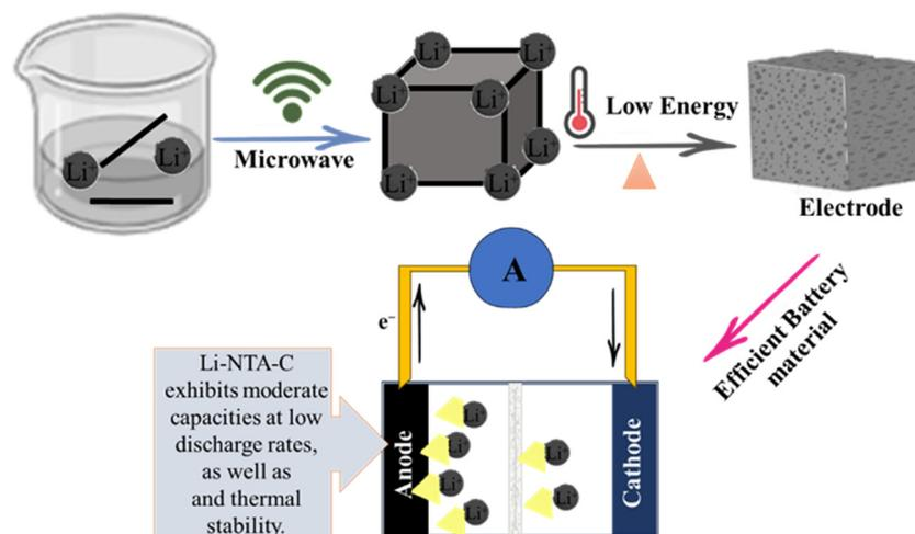
Fig. 5 The application of MOFs in lithium ion batteries.<sup>108</sup>
