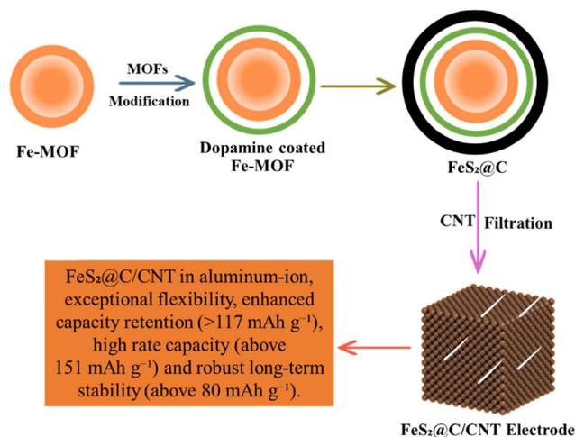
Fig. 10 The application of MOFs in aluminum air batteries.<sup>157</sup>
