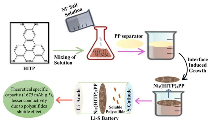
Fig. 6 The application of MOFs in lithium sulfur batteries.<sup>116</sup>
