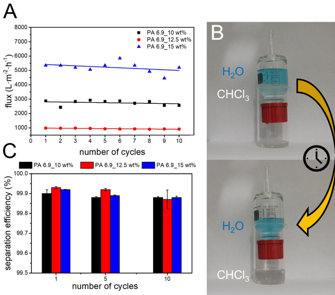
**Fig. 6** Results for the separation of water and chloroform, (A) the initial permeate flux for each separation cycle (linear fit), (B) filtration setup with a mixture of chloroform and water before and after filtration, (C) separation efficiency during the first, fifth and tenth cycle.
