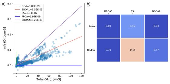
Fig. 4 (a) Concentrations of m/z 60 against concentrations of total OA at COALA, superimposed with lines that use  $f_{60}$  of each factor from the COALA 5-factor PMF solution as their gradient. Values of  $f_{60}$  for each factor are quoted in the legend; (b) Spearman's  $\rho$  coefficients between the concentrations of PMF factors from the COALA 5-factor solution that contain m/z 60 (BBOA1, sea salt, and BBOA2) with levoglucosan (top) and radon (bottom).
