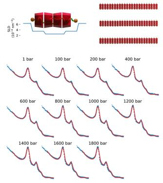
Fig. 2 Top: Scattering length density profile and schematic representation of the layer cross-section and schematic representation of the multilayered structure. Bottom, SANS scattering intensities from  $\alpha$ CD-C<sub>12</sub>E<sub>5</sub>CH<sub>2</sub> COONa complexes at different hydrostatic pressure values. Solid lines are best fits according to a model of stacked membranes, as described in the text. For absolute intensities and scattering vector values refer to Fig. 1.
