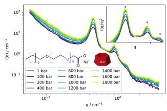
Fig. 1 Small-angle neutron scattering data from a αCD-C<sub>12</sub>E<sub>5</sub>CH<sub>2</sub> COOH complexes as a function of the applied hydrostatic pressure. Inset shows region at mid-q with the correlation peaks stemming from the multilayered order within the aggregates in a  $I(q) \cdot q^2$  vs. q representation for improved readibility. Peak positions of  $q^* = [0.45, 0.90, 1.35]$  nm<sup>-1</sup> are
