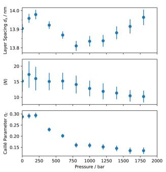
Fig. 3 Structural obtained from the fit of the pressure dependent SANS data from  $\alpha$ CD-C<sub>12</sub>E<sub>5</sub>CH<sub>2</sub> COO Na complexes. From top to bottom: the interlayer spacing, the average number of aggregate involved in one multilayered aggregate, and the Caillé parameter, related to the membrane stiffness. Error bars result from the uncertainty determined from the least squares minimization procedure.
