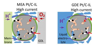
Fig. 4 Schematic illustration of oxygen transport being affected by the ionic liquid modification of Pt/C in the high current density regime in MEA (left) and GDE (right)
