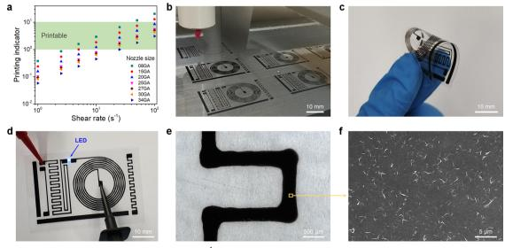
Fig. 4 (a) Printing indicator of the graphene inks (10 mg mL<sup>-1</sup>) at different shear rates. (b) Printing of multiple flexible conductive circuit patterns. (c) Bending of the printed flexible conductive circuit without failure. (d) Lighting up of an LED chip on the printed flexible conductive circuit. (e) The optical microscopy image of a printed line. (f) The corresponding SEM image of the printed pattern.
