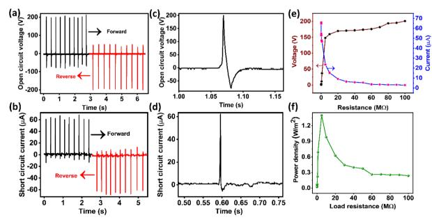
Fig. 2 Electrical characteristics of the X-TENG (5  $\times$  5 cm<sup>2</sup>), (a)  $V_{oc}$  in forward and reverse connections and (b)  $I_{sc}$  in forward and reverse connections, (c) and (d) enlarged views of  $V_{oc}$  and  $I_{sc}$  in one complete cycle, (e) X-TENG output voltage and current as a function of various load resistances, and (f) instantaneous power density with the load resistance.
