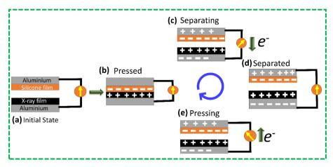
Fig. 3 Working mechanism of the X-TENG at (a) initial state, (b) pressed state, (c) separating state, (d) completely separated state, and (e) pressing state.
