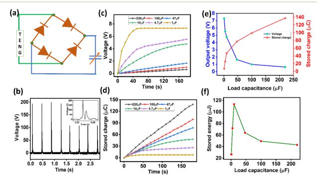
Fig. 6 (a) Schematic of the X-TENG output rectification, (b) TENG output after rectification; the inset shows a magnified view of one cycle output, (c) charging curves of different load capacitors, (d) stored charge at different load capacitances, (e) output voltage and stored charge behaviour as a function of the load capacitance, and (f) the maximum stored energy as a function of the load capacitance.
