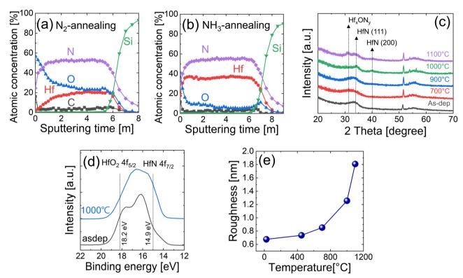
Fig. 4 AES depth profile of the HfN<sub>x</sub> film annealed at 900 °C with (a) N<sub>2</sub> and (b) NH<sub>3</sub> ambient. (c) Grazing-angle incidence X-ray diffraction (GIXRD) analysis of films annealed at various temperatures, X-ray photoelectron spectroscopy of films annealed at various temperatures, and (e) roughness. All films were deposited with the precleaning step, with a thickness of 15 nm, and annealing was conducted in NH<sub>3</sub> ambient, except for (a).
