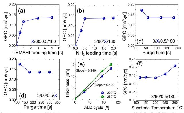
Fig. 2 Variation of growth per cycle (GPC) of HfN<sub>x</sub>, deposited with the precleaning step, with the change in (a) Hf[N(CH<sub>2</sub>)(C<sub>2</sub>H<sub>5</sub>)]<sub>4</sub> (TEMAHf) feeding time, (b) NH<sub>3</sub> feeding time, (c) TEMAHf purge time, and (d) NH<sub>3</sub> purge time. (e) Increasing thickness of HfN<sub>x</sub> film with ALD cycle at different temperature, and (f) change in HfN<sub>x</sub> GPC with increasing substrate temperature.
