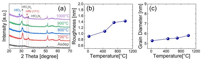
Fig. 6 (a) GIXRD, (b) roughness, and (c) grain diameter dependence on the annealing temperature of 15nm  $HfN_x$  films deposited without the precleaning step. All samples were annealed at  $NH_3$  ambient.
