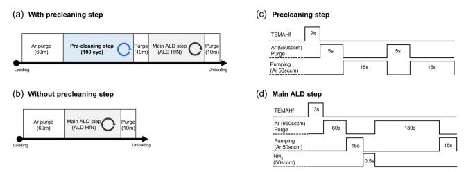
Fig. 1 Atomic layer deposition(ALD) process flow of HfN<sub>x</sub> from substrate loading to unloading, (a) with and (b) without the precleaning step. Pulse time and Ar flow of one cycle of (c) precleaning step and (d) main ALD step.
