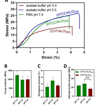
Fig. 8 Mechanical properties of the FS membranes in PBS (pH 7.4) and acetate buffer (pH 5.5). (A) Representative stress-strain curves, (B) Young modulus, (C) elongation-at-break, and (D) ultimate tensile strength. Data are presented as mean  $\pm$  SD of three independent experiments (n = 3, per condition) performed in triplicates. Significant differences were found for \*\*  $p \le 0.01$
