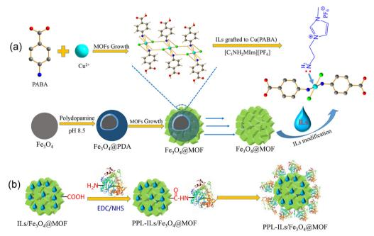
Scheme 1 (a) The synthesis route of ionic liquid modified Fe<sub>3</sub>O<sub>4</sub>@MOF and (b) schematic illustration of lipase covalent immobilization on ILs/ Fe<sub>3</sub>O<sub>4</sub>@MOF.
