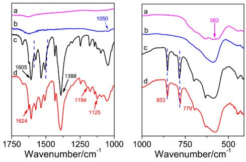
Fig. 1 FTIR spectra of (a) Fe<sub>3</sub>O<sub>4</sub>, (b) Fe<sub>3</sub>O<sub>4</sub>@PDA, (c) Fe<sub>3</sub>O<sub>4</sub>@MOF, and (d) ILs/Fe<sub>3</sub>O<sub>4</sub>@MOF.
