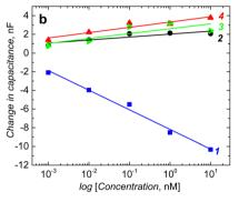
Fig. 6 (a) Measurement of the change in the capacitance of the semicovalently surface imprinted macroporous MIP film in the presence of (1) BSA, (2) HSA, (3) myoglobin, and (4) cytochrome c before post-imprinting modification and (b) corresponding calibration curves. Measurement was performed in 10 mM MES buffer (pH = 4.2). Potential: 0.2 V; frequency: 10 Hz.
