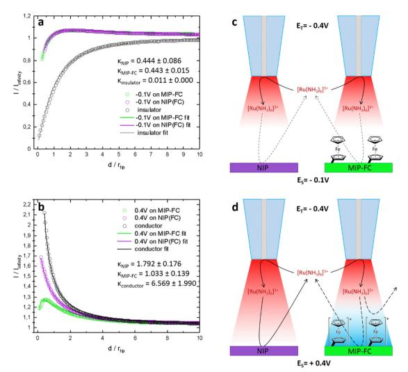
Fig. 7 SECM studies performed in feedback mode. Approach curves recorded on post-imprinting modified and non-imprinted macroporous film samples biased at (a) -0.1 V and (b) 0.4 V vs. Ag<sub>pseudo</sub>. Schemes showing post-imprinted and non-imprinted macroporous film behavior at (c) -0.1 V and (d) +0.4 V biased potential.  $E_S$ -potential applied to the sample electrode,  $E_T$ -potential applied over Pt microelectrode tip.
