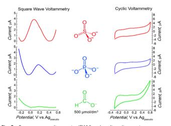
Fig. 2 Square wave voltammetry (SWV) and cyclic voltammetry measurement on the electrode coated with 3,3'-bithiophene (CR2) and p-bis(2,2'bithien-5-yl)methylbenzoic acid (FM2) copolymers, after modification with aminoferrocene, performed in the 0.5 mM aqueous solution of H<sub>2</sub>SO<sub>4</sub>, or H<sub>3</sub>PO<sub>4</sub> or HCOOH. SWV measurement conditions: pulse height: 25 mV, pulse width: 50 ms, step height: 10 mV, CV: 50 mV s<sup>-1</sup>.
