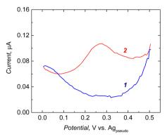
Fig. 1 Electrochemical measurement performed at the electrode coated with 3,3'-bithiophene (CR2) and p-bis(2,2'-bithien-5-yl)methylbenzoic acid (FM2) co-polymers (1) before and (2) after its modification with aminoferrocene. DPV measurement conditions: pulse height: 2.5 mV, pulse width: 100 ms, step height: 5 mV, step time 500 ms, 0.1 M LiClO<sub>4</sub>/
