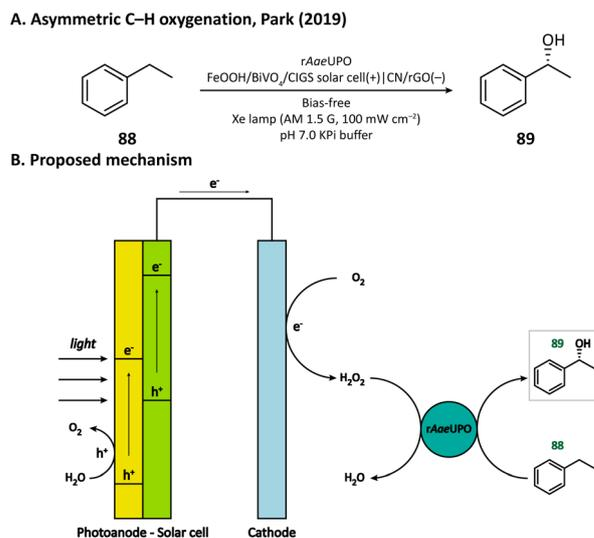
Fig. 14 Cathode-mediated *in situ* H<sub>2</sub>O<sub>2</sub> generation for asymmetric C–H oxygenation.
