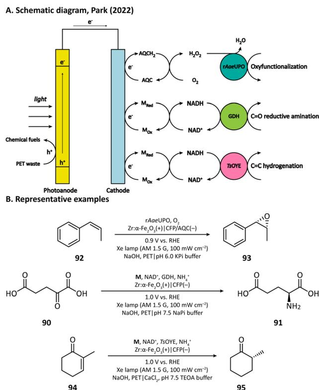
Fig. 16 PET conversion coupled with cathode-mediated biosynthesis.
