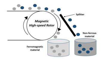
Fig. 3 Schematic representation of a magnetic separator (adapted from Hsu et al., 2019).
