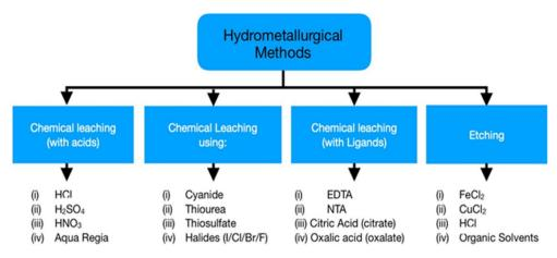
Fig. 6 Hydrometallurgical processes
