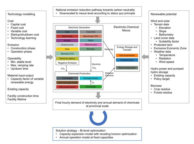
Fig. 1 Framework of the proposed nexus optimization model.
