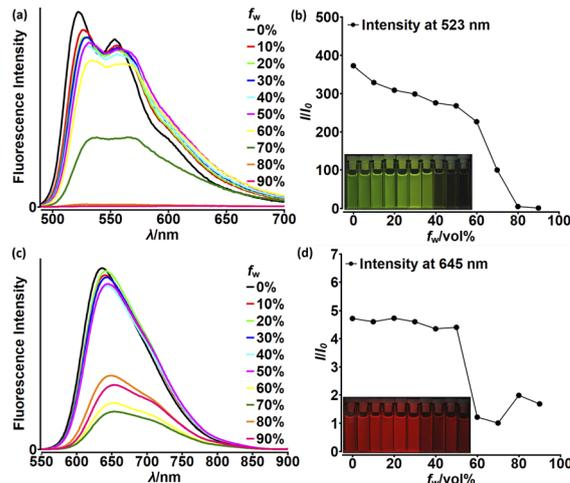
Fig. 10 Fluorescence spectra of **1c** (a) and **46** (c) in THF–water mixtures of different relative proportions. Plots of maximum intensity vs. % water fraction ( $f_w$ ) for dyes **1c** (b) and **46** (d). Insets: photographs of **1c** (b) and **46** (d) in THF–water mixtures with different water fractions under UV illumination (0% to 90% water fraction from left to right). Dye concentration:  $\sim 10$  mM. Adapted with permission from ref. 30c. Copyright 2018 Royal Society of Chemistry.
