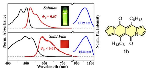
Fig. 14 Normalized absorption (black) and fluorescence (red) spectra of DPND in CH<sub>2</sub>Cl<sub>2</sub> solution (10<sup>-5</sup> M) and solid thin film (100 nm), as well as sensitized phosphorescence spectra (blue) of 1h in polystyrene (PS) matrix (DPND : PtTPBP : PS = 1 : 5 : 94) and doped thin film (DPND : PtTPBP = 95 : 5). Inset: sample photographs of solution and thin film under 365 nm UV light. Adapted with permission from ref. 8d. Copyright 2020 American Chemical Society.
