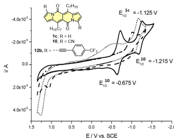
Fig. 8 Cyclic voltammograms of the dyes **1c** (dotted line), **10** (solid line) and **12b** (dashed line) in dichloromethane measured using the saturated calomel electrode (SCE) as the reference. Adapted with permission from ref. 18 Copyright 2016 Royal Society of Chemistry.
