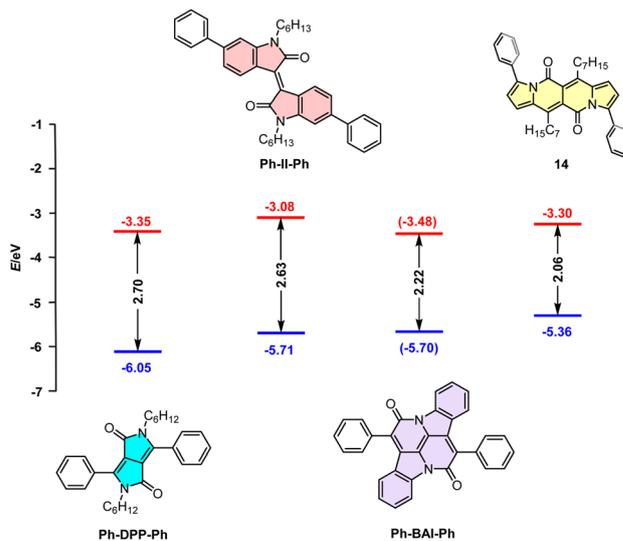
**Fig. 13** Correlation diagram of the HOMOs and LUMOs of three representative cross-conjugated units and a DPND derivative **14** determined by cyclic voltammetry (CV) measurements in CH<sub>2</sub>Cl<sub>2</sub> (the values in parentheses were determined using DFT calculations due to lack of the experimental data).
