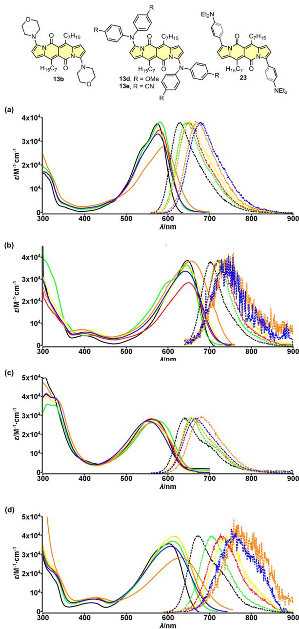
Fig. 6 Absorption (solid) and emission (dotted) spectra of compounds **13b** (a), **13d** (b), **13e** (c) and **23** (d) measured in cyclohexane (black), toluene (green), THF (red),  $\text{CH}_2\text{Cl}_2$  (yellow), MeCN (blue) and DMSO (orange). Adapted with permission from ref. 28 Copyright 2018 American Chemical Society.
