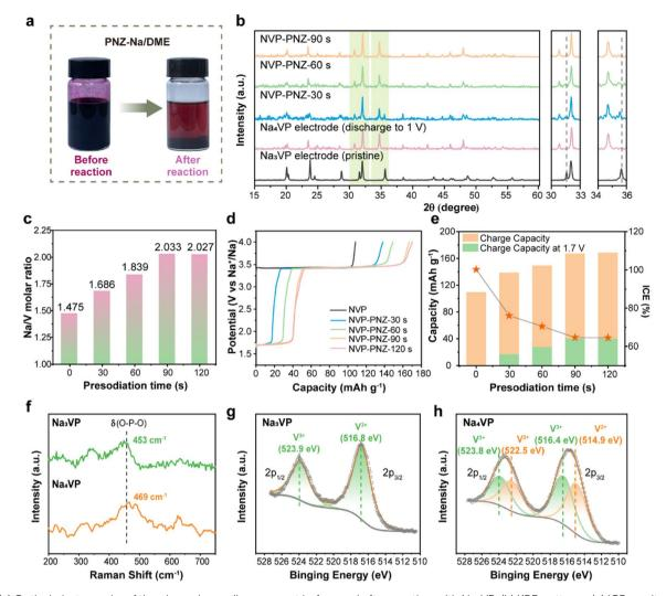
Fig. 2 (a) Optical photographs of the phenazine sodium reagent before and after reaction with  $Na_3VP$ . (b) XRD patterns, (c) ICP results, (d) initial charge curve, and (e) initial charge capacity and ICE of the  $Na_3VP$  electrodes with different presodiation times. (f) Raman spectroscopy spectra of  $Na_3VP$  and  $Na_4VP$ . XPS V 2p spectra of (g)  $Na_3VP$  and (h)  $Na_4VP$ .
