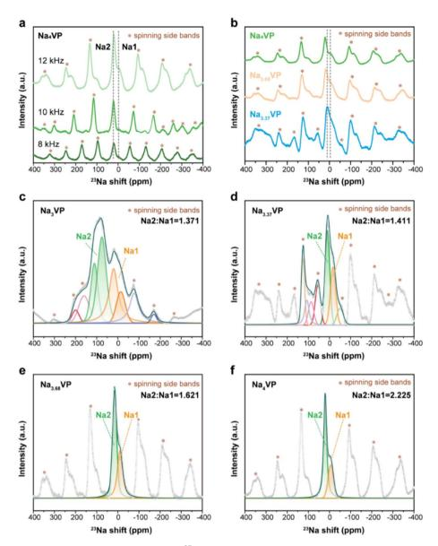
Fig. 4 (a)  $^{23}$ Na ssNMR spectra of Na<sub>4</sub>VP at 8, 10, and 12 kHz. (b)  $^{23}$ Na ssNMR spectra of Na<sub>2</sub>VP with different sodiation depths at 12 kHz. The fitted  $^{23}$ Na ssNMR spectra of (c) Na<sub>3</sub>VP, (d) Na<sub>3,37</sub>VP, (e) Na<sub>3,68</sub>VP, and (f) Na<sub>4</sub>VP.
