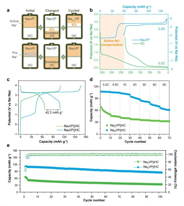
Fig. 6 (a) Schematic illustration of the presodiation process by the Na-enriched Na<sub>4</sub>VP cathode in full cells. (b) Half-cell voltage profiles of the Na<sub>4</sub>VP cathode and the HC anode at 0.2C. (c) Initial voltage profiles, (d) rate performance, and (e) cycling stability at 1C of Na<sub>3</sub>VP||HC and Na<sub>4</sub>VP||HC full cells.
