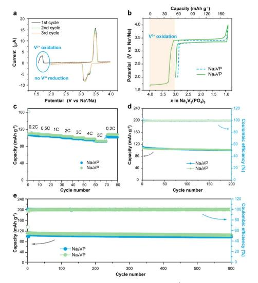
Fig. 5 (a) Cyclic voltammogram profiles of the Na<sub>4</sub>VP cathode at a scan rate of  $0.1 \text{ mV s}^{-1}$ . (b) Initial charge-discharge curves of Na<sub>3</sub>VP and Na<sub>4</sub>VP electrodes between 2.0 and 4.0 V at 0.2C. (c) Rate performance, (d) cycling stability at 0.5C, and (e) long-term cycling stability at 1C of Na<sub>3</sub>VP and Na<sub>4</sub>VP electrodes
