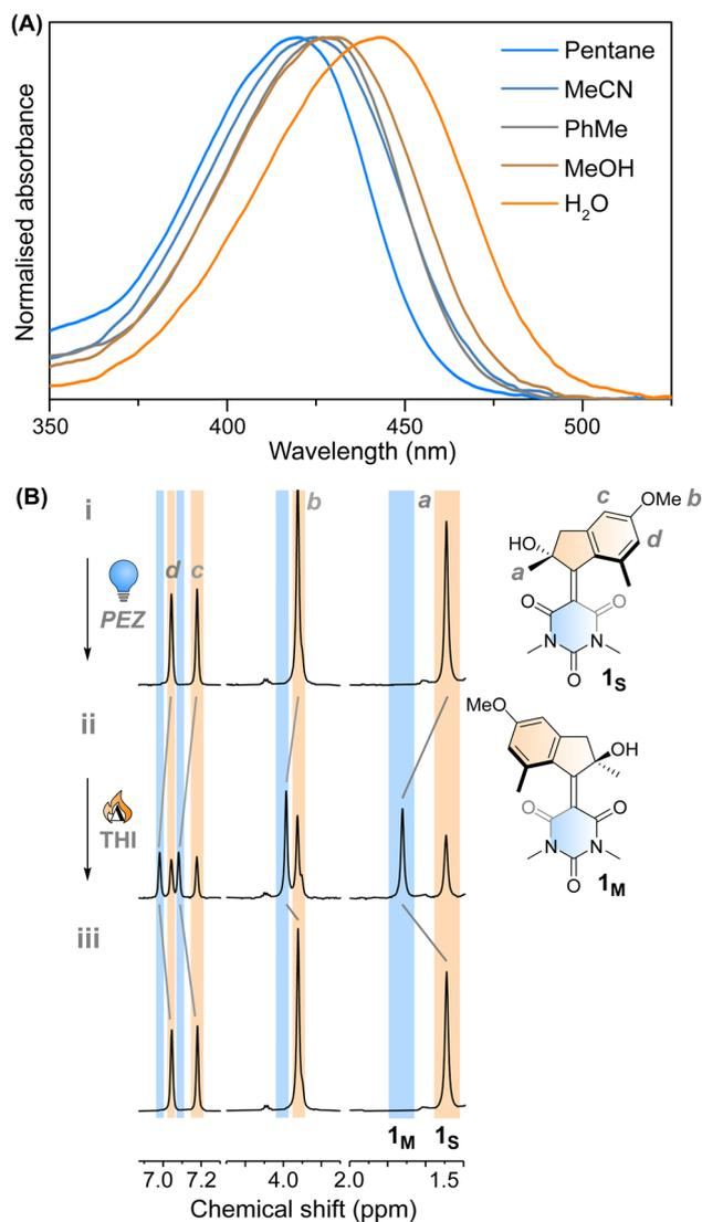
Fig. 2 (A) Normalised UV-vis absorption spectra of  $1_s$  in different solvents. (B)  $^1\text{H}$  NMR irradiation studies of  $1_s$  in  $\text{CD}_3\text{OD}$  ( $c = 1 \times 10^{-3}$  M) at  $-90$  °C. (i)  $1_s$  before irradiation; (ii)  $\text{PSS}_{420}$ , 63 : 37 ( $1_M$  :  $1_s$ ); (iii) THL,  $-45$  °C, 15 min.
