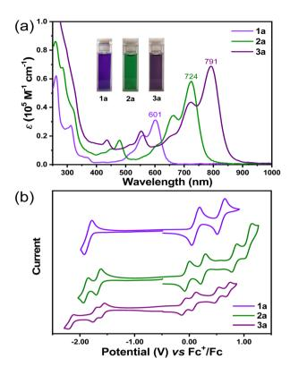
Fig. 3 (a) UV-vis spectra of 1a, 2a and 3a in dichloromethane  $(1 \times 10^{-5} \text{ M})$ , inset are the photos of their solutions. (b) Cyclic voltammograms of 1a, 2a and 3a (V vs. Fc<sup>+</sup>/Fc, in 0.1 M nBu<sub>4</sub>N·PF<sub>6</sub>/dichloromethane).
