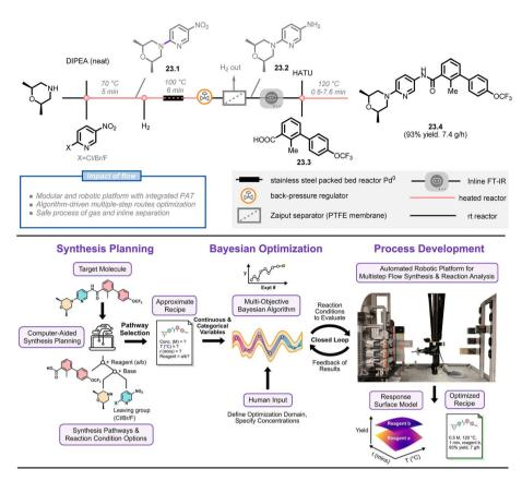
Fig. 23 Overall approach for bayesian optimization algorithm-driven multistep-synthesis of Sonidegib on an automated robotic platform. DIPEA: N,N-diisopropylethylamine, HATU: hexafluorophosphate azabenzotriazole tetramethyl uronium. Reproduced from ref. 150 with the permission of American Chemical Society, copyright 2022.
