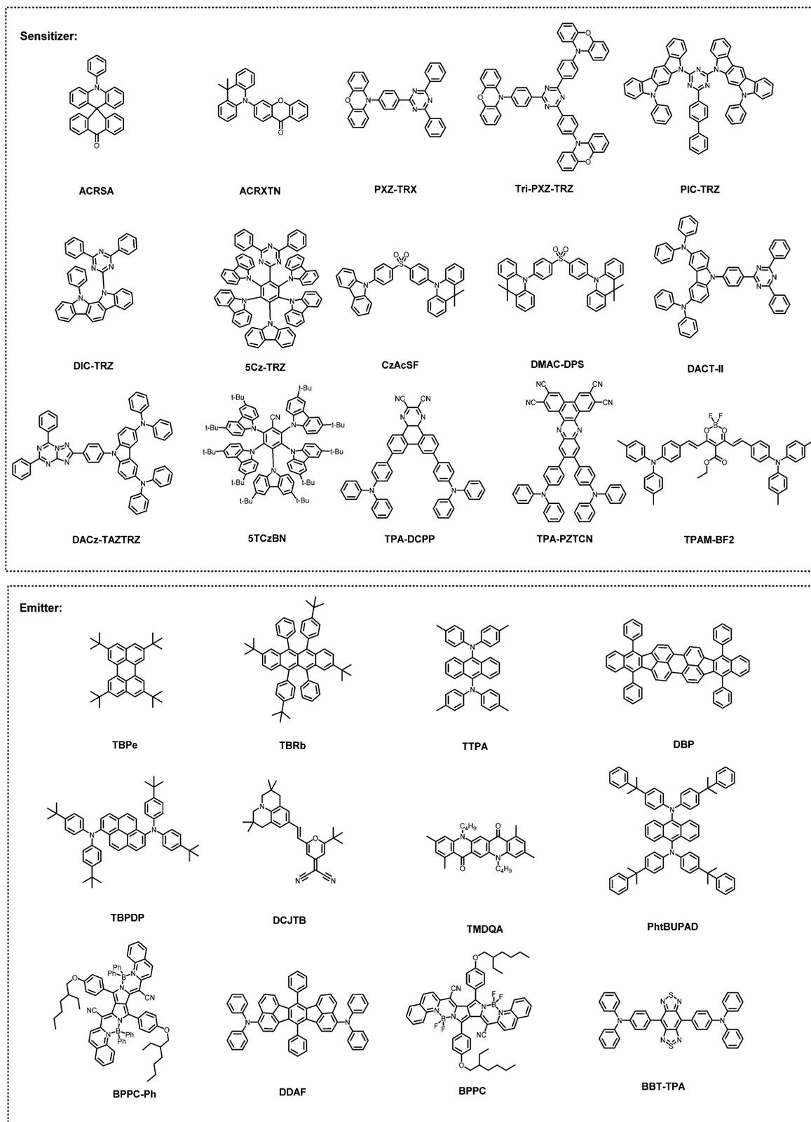
Fig. 6 Chemical structures of TADF sensitizers and fluorescent emitters.
