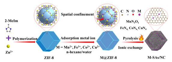
Scheme 1 Schematic illustration of the synthesis process of metal-N<sub>x</sub> species embedded in the porous N-doped porous carbon (M-SAs/NC) composite. Brown, purple, red, and white balls represent C, metal atoms, O, and N, respectively.
