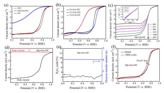
Fig. 5 ORR performance in 0.5 M H<sub>2</sub>SO<sub>4</sub> solution. (a and b) LSV curves of various catalysts at a rotating speed of 1600 rpm. (c) LSV curves and K-L plots (the inset) of Mn-SAs/NC at different rotating rates. (d) RRDE measurements of Mn-SAs/NC and (e) the corresponding electron transfer number and H<sub>2</sub>O<sub>2</sub> yield. (f) The LSV curves before and after the CV cycling test for Mn-SAs/NC.
