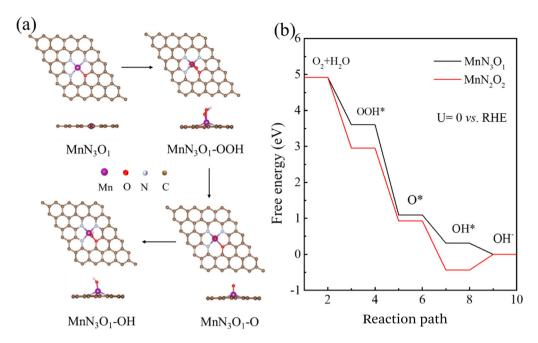
Fig. 6 Top and side views of the optimized adsorption model of O\*, OH\*, and OOH\* on  $MnN_3O_1$ . Brown, purple, red, and white balls represent C, Mn, O, and N, respectively. (b) Under the condition of U = 0 V, the  $4e^-$  association pathway at the active site of  $MnN_3O_1$  and  $MnN_2O_2$  calculates the free energy evolution of the ORR.
