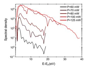
Fig. 5 Energy spectra for V = 100 V under laser illumination varying the intensity from 12 GW cm<sup>-2</sup> (red) to 25 GW cm<sup>-2</sup>.
