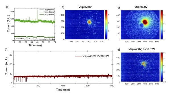
Fig. 2 (a) Short term stability for three values of the extracting voltage. (b) FEM patters for DC field emission at V = 600 V; (c) FEM pattern for DC field emission at V = 800 V; (d) long-term stability for multiphoton photoemission at the extraction voltage of 400 V and laser intensity of  $2.8 \times 10^{10} \text{ W cm}^{-2}$ . (e) FEM pattern, for the emission reported in (d).
