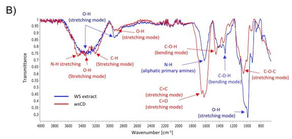
Fig. 2 Chemical structure and surface functional group analysis. (A) Chemical structure analysis of WS extract and wsCDs using UV absorption spectroscopy; (B) surface functional group analysis of WS extract (blue) and wsCDs (red) using Fourier transform infrared spectroscopy.
