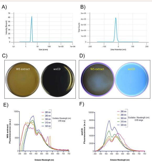
Fig. 1 Physicochemical analysis of wsCDs and WS extract. (A) Particle size distribution of carbon dots; (B) zeta potential of carbon dots; (C) image of WS extract and wsCDs under white light; (D) photoluminescence of WS extract and wsCDs under UV excitation; (E) fluorescence emission scan of WS extract at varying UVB excitation wavelengths; (F) fluorescence emission scan of wsCDs at varying UVB excitation wavelengths.
