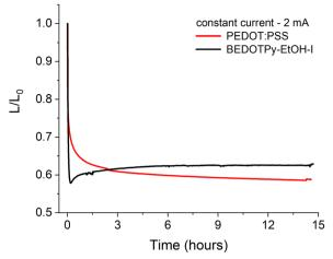
Fig. 7 Lifetime studies of OLEDs containing dimerised and doped BEDOTPy-EtOH-I and PEDOT:PSS as the hole transport layer. Lifetime measured by the luminance (L) divided by the initial luminance (L<sub>0</sub>). Device structure ITO/HTL/Super Yellow/Ca/Al; OLEDs held at a constant current of 2 mA for approx. 14 hours, with luminance measurements every minute.
