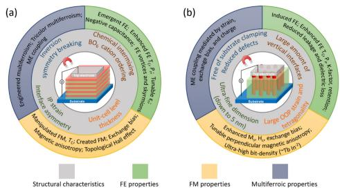
Fig. 1 Schematic diagrams showing structural characteristics (inner ring) and observed interface-related phenomena (outer ring) in epitaxial ferroic thin films formed from (a) SL structures and (b) VAN structures. Tricolor multiferroism is a kind of multiferroism induced in a three-component SL. See Fig. 2-8 for more details about how both structural and physical effects link to the observed interface-related phenomena
