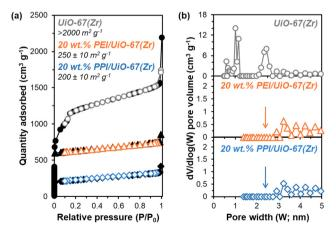
Fig. 3 (a) Adsorption-desorption isotherms (77 K) and (b) NLDFT pore size distributions from N<sub>2</sub> physisorption for UiO-67(Zr) (grey circles), 20 wt% PEI/UiO-67(Zr) (orange triangles), and 20 wt% PPI/UiO-67(Zr) (blue diamonds). Isotherms for 20 wt% PEI/UiO-67(Zr) and 20 wt% PPI/UiO-67(Zr) are shifted vertically for clarity
