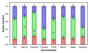
Fig. 6 Primary (red), secondary (green), and tertiary (blue) amine distributions for as-synthesized poly(propylene imine) after exposure to different solvent environments of varying polarity (white circles) at ambient temperature (298 K) for 8 h. Distributions are determined via <sup>1</sup>H NMR in D<sub>2</sub>O solvent
