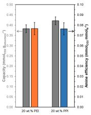
Fig. 8 Amine efficiencies (orange, blue) and mass-normalized CO<sub>2</sub> capacities (grey) at 308 K for 20 wt% PEI/UiO-67(Zr) (orange) and 20 wt% PPI/ UiO-67(Zr) (blue) from 40 mL min<sup>-1</sup> simulated air (400 ppm CO<sub>2</sub> in He) after 3 h under 40 mL min<sup>-1</sup> Ar at 383 K.
