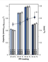
Fig. 2 Mass-normalized CO<sub>2</sub> capacities for varying weight percentages (20-50) of PPI supported on UiO-67(Zr) for three 1 h uptake cycles at 308 K from simulated flue gas with 2 h regeneration steps at 383 K under 40 mL min<sup>-1</sup> Ar flow in between cycles.  $t_{20}$  (circles) are times to reach 20% of equilibrium CO2 uptakes.
