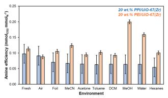
Fig. 4 Amine efficiencies (mmol<sub>CO<sub>2</sub></sub> mmol<sub>N</sub><sup>-1</sup>) determined from 1 h CO<sub>2</sub> uptakes at 308 K from simulated flue gas for 20 wt% PPI/UiO-67(Zr) (blue) and 20 wt% PEI/UiO-67(Zr) (orange) after 7 days of exposure to each solvent environment. Amine contents are based on molecular weights of 400 g mol<sup>-1</sup> for PPI (77% primary and secondary amines) and 800 g mol<sup>-1</sup> for PEI (77% primary and secondary amines). 36,37
