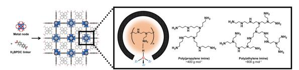
Fig. 1 Zr<sub>6</sub>O<sub>4</sub>(OH)<sub>4</sub> nodes and biphenyl-4,4'-dicarboxylic acid linker species that form the UiO-67(Zr) nanoporous framework structure containing larger octahedral and smaller tetrahedral cages that can host aminopolymer (poly(propylene imine) and poly(ethylene imine)) guests, which serve as CO<sub>2</sub> adsorption sites.
