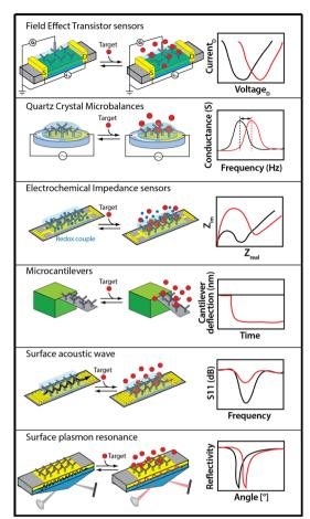
**Fig. 3** Approaches that monitor the adsorption of the target to a receptor-coated surface *via* the associated change in charge, mass, steric bulk, or optical properties may prove suitable for the development of measure-and-act LOC technologies.
