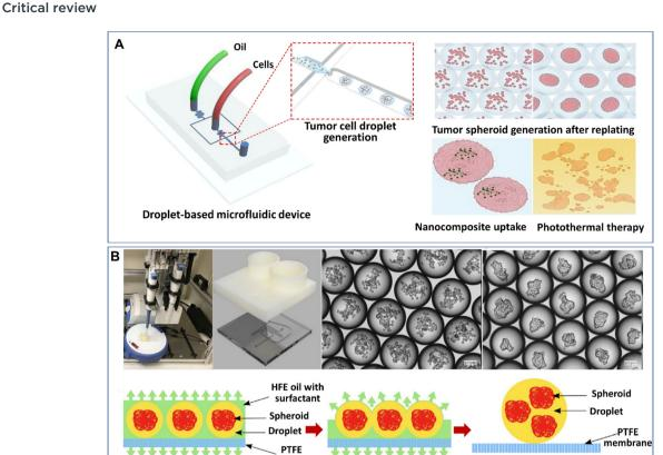
Fig. 2 Formation of spheroids in liquid droplets by droplet microfluidics. (A) Spheroids formed in liquid droplets and used for photothermal therapy testing. Reproduced from ref. 53 with permission from Springer Nature, copyright 2020. (B) Spheroids formed in an automated droplet generator and recovered on a hydrophobic membrane. Reproduced from ref. 54 with permission from the Society for Laboratory Automation and Screening, copyright 2020.
