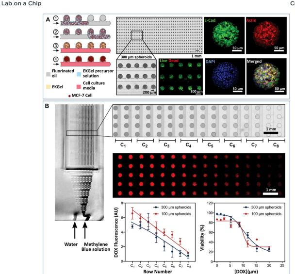
Fig. 7 Formation of tumour spheroids and drug efficacy test in a 2D array DMF platform. (A) Tumour spheroids formed from the self-digitization of cells in a hydrogel suspension into fluorinated oil. (B) Cytotoxicity test of drugs in a concentration-gradient generator. Scale bars are 1 mm. (A) and (B) were reproduced from ref. 128 with permission from John Wiley & Sons Inc, copyright 2021.
