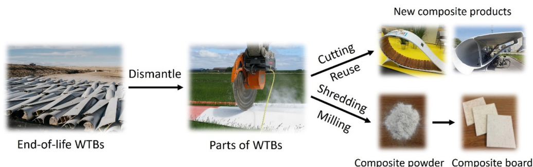
Fig. 4 Mechanical recycling processes of end-of-life WTBs.
