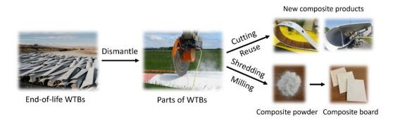
Fig. 4 Mechanical recycling processes of end-of-life WTBs.
