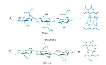
Fig. 15 Chemical structure and possible intermolecular hydrogen bonding (--) in (a) chitin and (b) chitosan.
