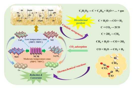
Fig. 8 Possible microthermal catalytic aerogenesis and metals conversion mechanism of BMW using waste NCM and its derivants as catalysts through thermochemical reactions.
