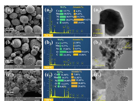
Fig. 6 SEM image, TEM image and corresponding EDS analysis of various elements in (a). Spent cathode material; (b). Roasted product at 500 °C, 15 min, NCM/BMW = 1:0.3; (c). Roasted product at 700 °C, 15 min, NCM/BMW = 1:0.3.
