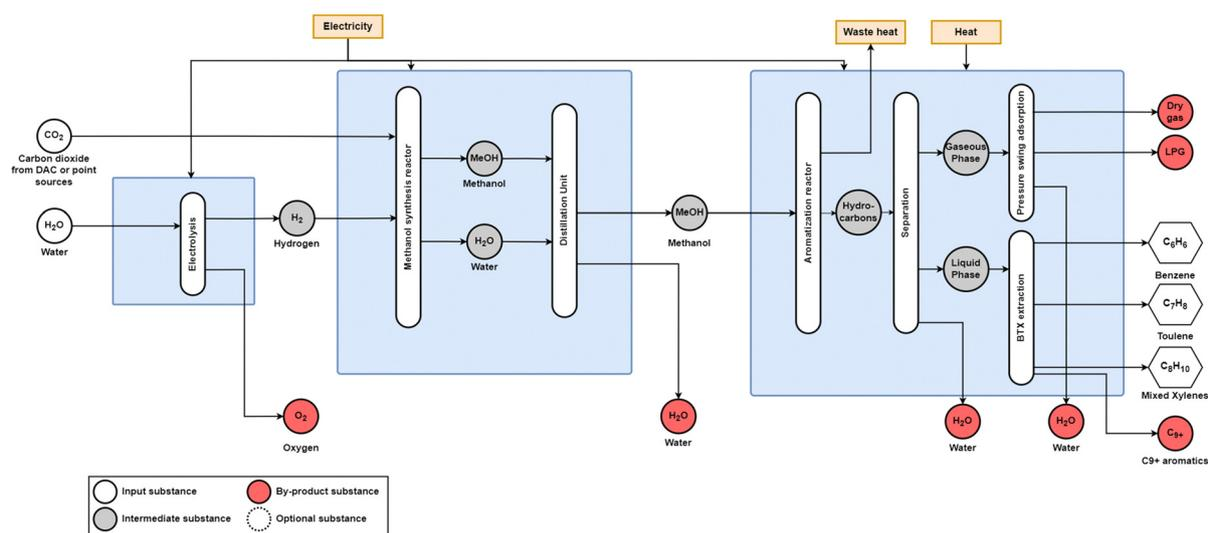
Fig. 14 Power-to-methanol-to-aromatic process diagram. Methanol synthesis occurs over a  $\text{CuOZnO}/\text{Al}_2\text{O}_3$  catalyst, and methanol aromatisation occurs over a HZSM-5 catalyst. Adapted from Jiang *et al.*<sup>26</sup>
