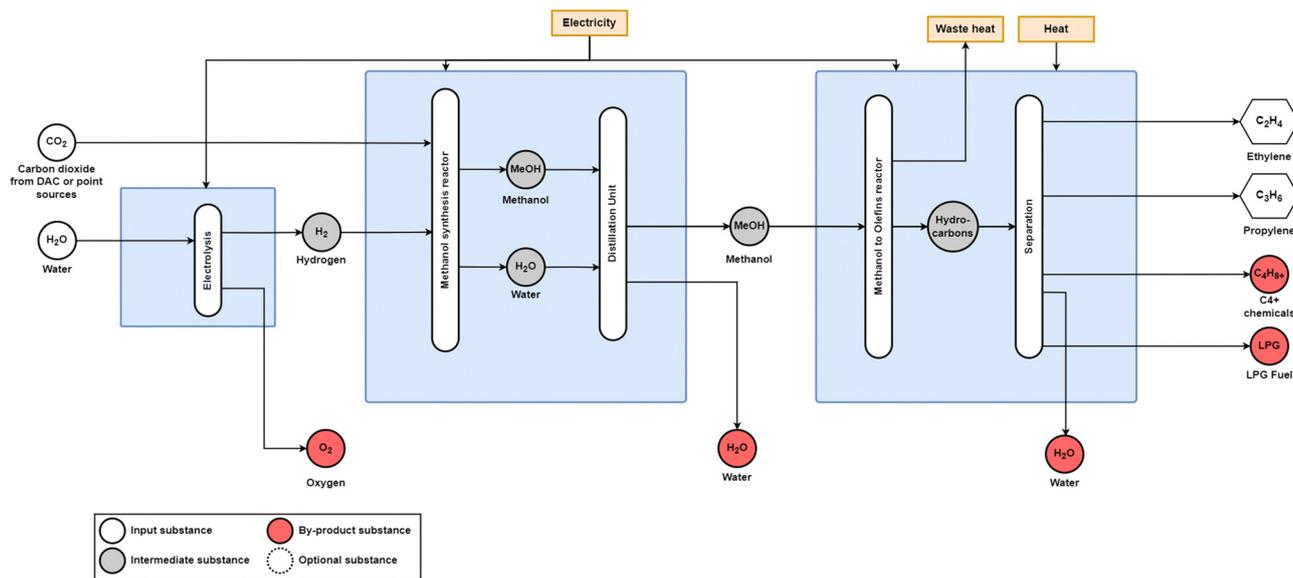
Fig. 13 Power-to-methanol-to-olefins process diagram. Methanol synthesis occurs over a  $\text{CuOZnO}/\text{Al}_2\text{O}_3$  catalyst and the MTO reactor uses the SAPO-34 catalyst. Adapted from Jiang *et al.*<sup>25</sup> and Dimian and Baldea.<sup>75</sup>
