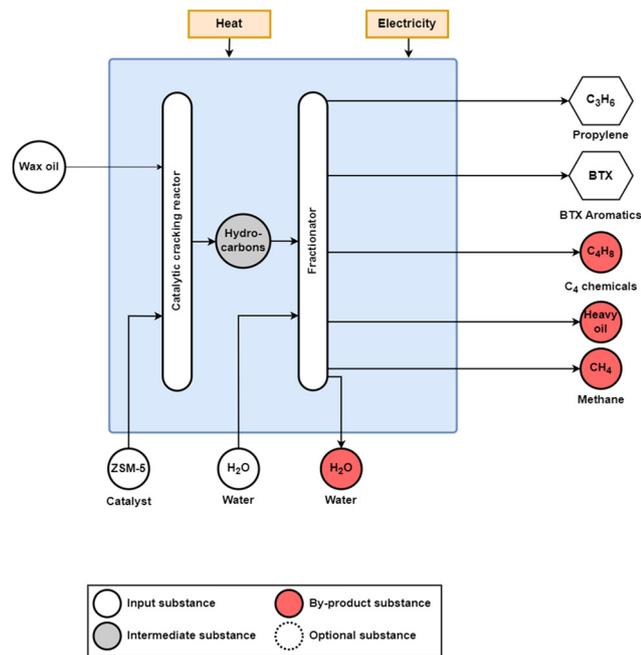
Fig. 5 Deep catalytic cracking of refinery oil for propylene production from wax oil using a zeolite (ZSM-5) catalyst. In addition to the propylene and BTX products, C<sub>4</sub> chemicals, heavy oil, and methane are also produced. Adapted from Zhao *et al.*<sup>24</sup> and Gholami *et al.*<sup>27</sup>
