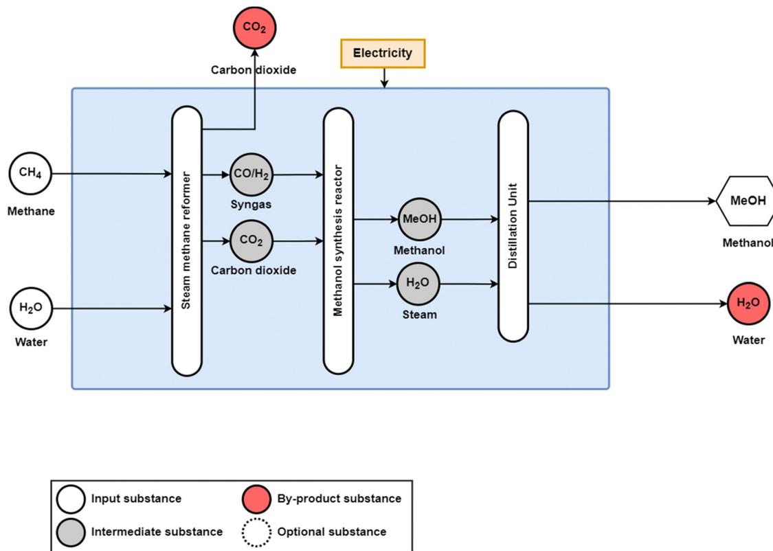
Fig. 2 Conventional production process for methanol synthesis from natural gas over a  $\text{CuO}/\text{ZnO}/\text{Al}_2\text{O}_3$  catalyst. Coal and oil can similarly be used as fossil feedstocks for coal gasification and partial oxidation for syngas production, respectively. Adapted from Adnan and Kibria.<sup>20</sup>
