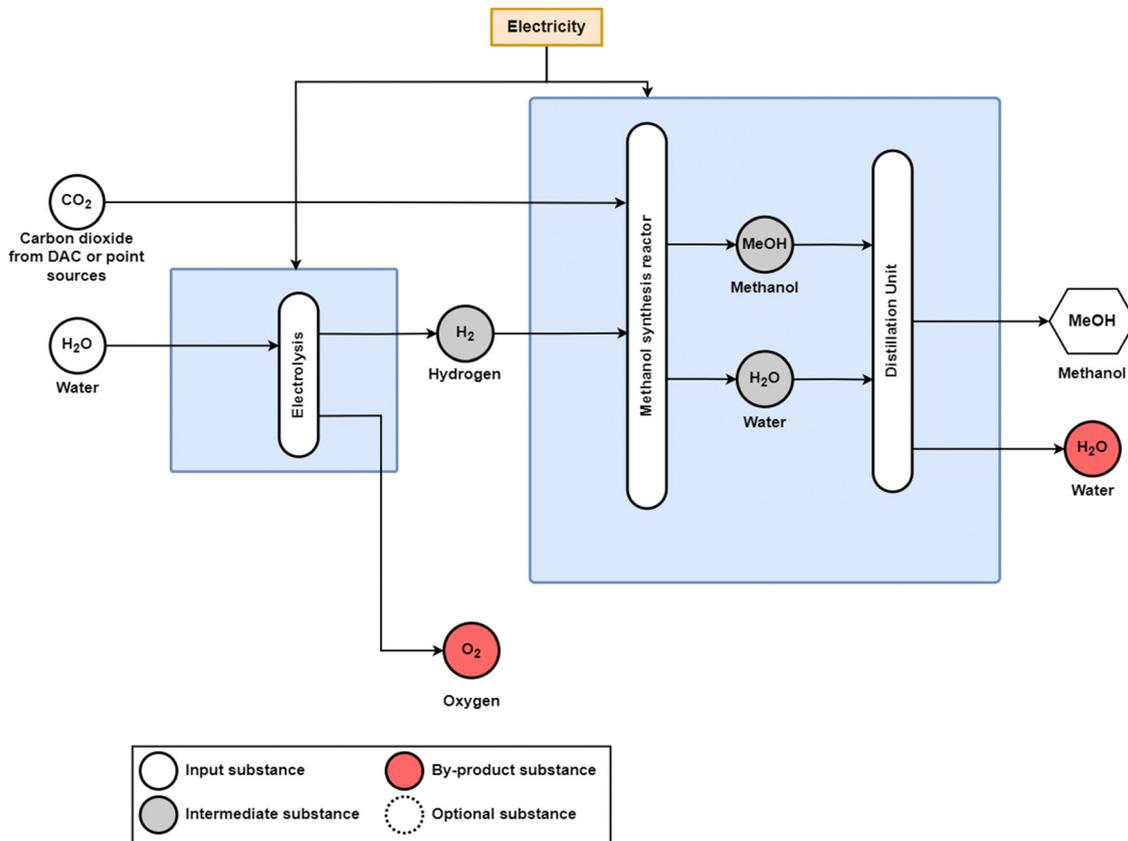
Fig. 12 Power-to-methanol process diagram with e-hydrogen supplied by water electrolysis and CO<sub>2</sub> being supplied by direct air capture (DAC) or industrial point sources. In this study, CO<sub>2</sub> from DAC is assumed. The catalyst for the methanol synthesis reactor is CuO/ZnO/Al<sub>2</sub>O<sub>3</sub>. Adapted from Adnan and Kibria<sup>20</sup> and Bos *et al.*<sup>64</sup>
