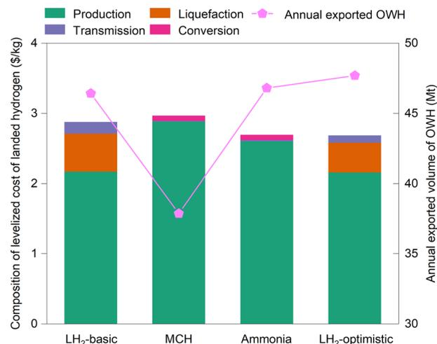
**Fig. 11** Comparison of average LCOH<sup>L</sup> and annual exported volume of OWH via liquid hydrogen, methylcyclohexane (MCH), and ammonia shipping in 2050.
