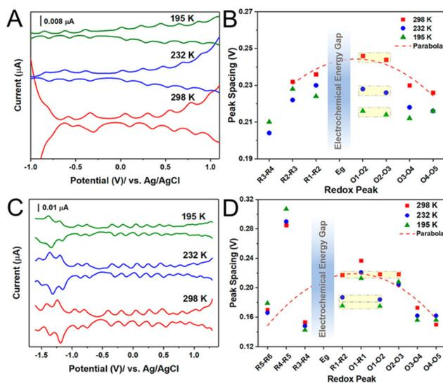
**Fig. 6** Temperature dependence of electrochemical properties of  $Au_{133}(TBBT)_{52}$  and  $Au_{144}(BM)_{60}$ . (A and C) The DPVs and (B and D) the electrochemical peak spacing of (A and B)  $Au_{133}(TBBT)_{52}$  and (C and D)  $Au_{144}(BM)_{60}$  at 298, 232, and 195 K. Peak spacing  $\Delta V$ s in (B) and (C) analyzed from (A) and (C), respectively. Reproduced with permission from ref. 97. Copyright 2020, American Chemical Society.
