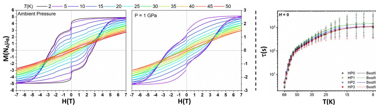
Fig. 2 Hysteresis loops of **1** at 2 K and 5–50 K in 5 K steps recorded at ambient pressure (left) and at 1 GPa (centre). For the series at 1 GPa, data below +/- 800 Oe at 5 K are omitted due to the superconductive manometer (Pb). Right: Relaxation profile ( $\tau$  vs.  $T$ ) for **1** at ambient pressure (HP0), 0.37 GPa (HP1), 0.79 GPa (HP2) and 1.2 GPa (HP3) (see Fig. S41 and S42, ESI<sup>†</sup> for fitted data and variations in the distribution of  $\tau$  ( $\beta$ ) with temperature).
