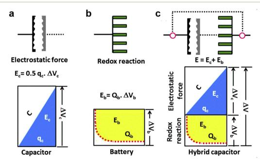
Fig. 3 Schematic representations of a single electrode system, (a) capacitor, (b) battery, and (c) hybrid capacitor according to the charge–potential profile with the corresponding equations for energy storage. Reproduced with permission from ref. 97. Copyright 2015, Royal Society of Chemistry.
