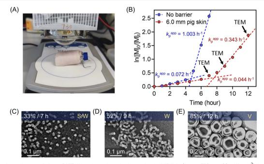
Fig. 7 (A) Experimental setup of photo-RAFT dispersion polymerization under the NIR light ( $\lambda_{max}=730$  nm; 60 mW cm<sup>-2</sup>) irradiation passing through 6.0 mm pig skin. (B) Comparison of dispersion photo polymerization kinetics between without barrier and through 6.0 mm pig skin. (C–E) Evolution of morphologies of polymeric nanoparticles synthesized through 6.0 mm pig skin indicated by corresponding TEM images at different time points (t=7, 9, and 12 hours).
