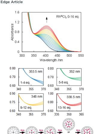
Fig. 1 Accumulation of Rh<sup>III</sup>Cl<sub>3</sub> to PPDPA16. (top) Change in UV-vis absorption spectra of PPDPA16 in DCM upon adding Rh<sup>III</sup>Cl<sub>3</sub> in MeCN/ MeOH = 250/1 up to 16 eq. ([PPDPA16] = ca. 5  $\mu$ M, 20 °C). (down) Enlarged views during complexation with Rh<sup>III</sup>Cl<sub>3</sub> in respective positions 0–4, 5–8, 9–12, and 13–16 eq. and the schematic illustration of the possible coordination sequence.
