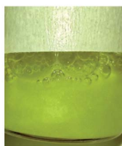
Fig. 3 (A) Size distribution of samples manufactured using 4% KP407 (in blue) and 4% TW20 (in orange). These samples were optically clear and likely contained quercetin solubilised within polymeric micelles. (B) Photograph of a sample prepared using 4% KP407. Quercetin did not precipitate in the form of crystals or nanoparticles, as it was likely solubilised within polymeric micelles. (C) Photograph of a sample prepared using 1% KP407. Quercetin precipitated in the form of coarse acicular crystals that sedimented at the bottom of the vial.
