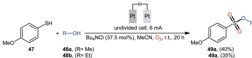
Scheme 23 Electrosynthesis of sulfonic esters **49** from 4-methoxybenzenethiol **47** and aliphatic alcohols **48** under O<sub>2</sub> atmosphere.
