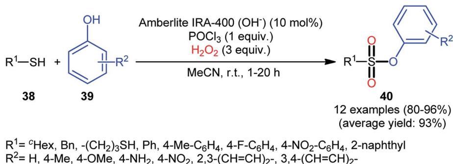
Scheme 18 Amberlite IRA-400/POCl<sub>3</sub>-mediated oxidative esterification of thiols **38** with phenols **39** in the presence of H<sub>2</sub>O<sub>2</sub>.
