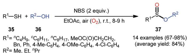
Scheme 17 NBS-mediated oxidative esterification of thiols **35** with alcohols **36**.
