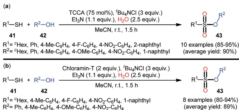
Scheme 19 (a) Hemmati's synthesis of sulfonic esters **43**; (b) Mojtahedi's synthesis of sulfonic esters **43**.
