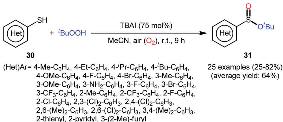
Scheme 13 TBAI-mediated oxidative esterification of (hetero)aromatic thiols **30** with <sup>*t*</sup>BuOOH developed by Zhang–Chen.
