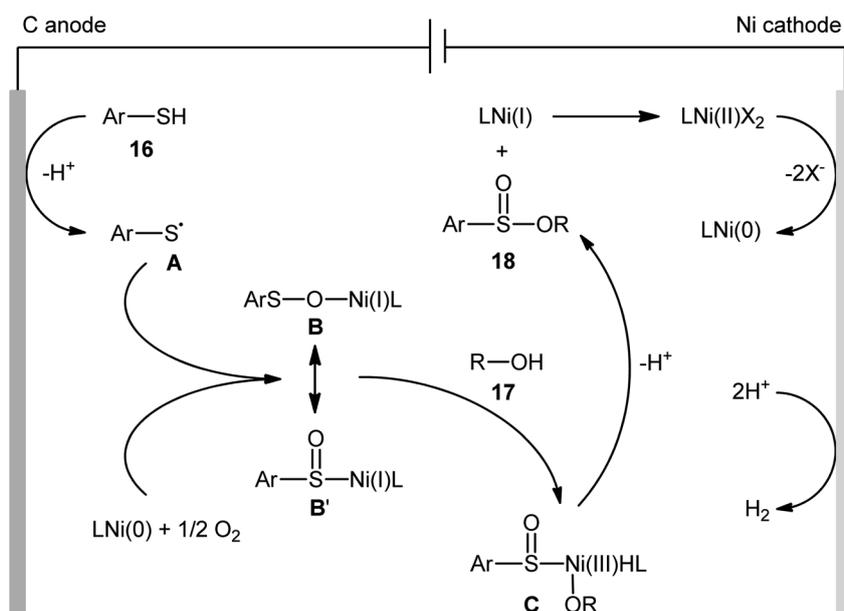
Scheme 7 Proposed mechanism for reaction in Scheme 6.
