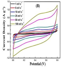
Fig. 6 (A) Comparison of the CV curves of single-walled nanotubes (SWNTs)/MnO<sub>2</sub> and SWNTs/MnO<sub>2</sub>/Ppy at a scan rate of 5 mV s<sup>-1</sup> (B) SWNTs/ MnO<sub>2</sub>/Ppy electrode CV curves at various scan rates. Reproduced from ref. 58 with permission from Elsevier, Copyright @ 2014.
