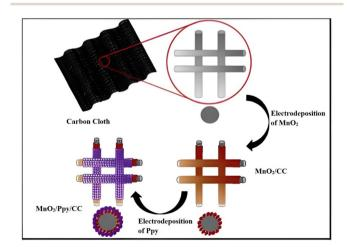
Fig. 2 Schematic view of the fabrication process of the flexible Ppy/ $MnO_2$  composite electrode. Reproduced from ref. 50 with permission from Elsevier, Copyright @ 2016.
