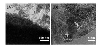
Fig. 3 (A) TEM image of the Ppy/MnO<sub>2</sub> nanocomposite; (B) highresolution TEM image of the Ppy/MnO<sub>2</sub> nanocomposite. Reproduced from ref. 50 with permission from Elsevier, Copyright @ 2016.
