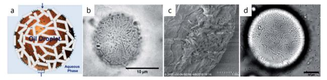
Fig. 6 Scheme of halloysite positioning onto the oil droplet (a), adapted from ref. 51 with permission from American Chemical Society, copyright 2015. Macondo crude oil halloysite emulsification, optical and cryo-SEM images (b and c), and A. borkumensis marine bacteria proliferation on the droplets after five days of exposure (d), (a) adapted from ref. 52 with permission from Elsevier, copyright 2018.
