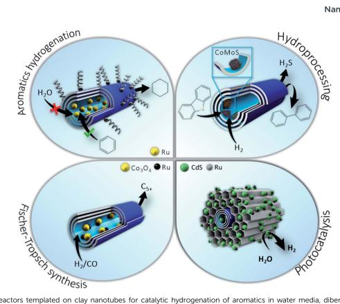
Scheme 5 Nanoreactors templated on clav nanotubes for catalytic hydrogenation of aromatics in water media, dibenzothiophene hydrodesulphurization, and Fischer-Tropsch synthesis and photocatalysis.
