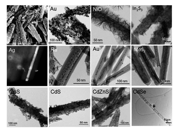
Fig. 2 Metal containing core—shell structures based on clay nanotubes, upper row – location outside: Aq, Au, NiO, and In<sub>2</sub>S<sub>3</sub> – taken from ref. 29 with permission, copyright by Elsevier, 2015. Middle row - tubes loaded inside: Aq, Ru, Au, and MoS2; bottom row - halloysite loaded inside/ outside: ZnS, CdS, CdZnS, and CdSe.
