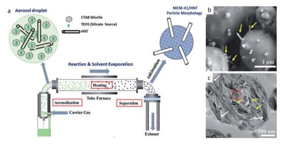
Fig. 4 Schematic illustration of the spray-drying technique (a), and SEM (b) and TEM (c) images of the resulting MCM-41/HNT particles. Adapted with permission from ref. 25 Copyright by American Chemical Society, 2022.
