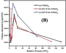
Fig. 4 (A) Nitrogen adsorption—desorption and (B) BJH pore diameter of pristine NiMnO<sub>3</sub>, 0.01 M Sm-doped NiMnO<sub>3</sub>, and 0.02 M Sm-doped NiMnO<sub>3</sub>.
