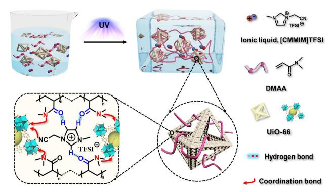
Scheme 1 Schematic of the preparation of UiO-66-ionogels. UiO-66 was mixed with N,N-dimethylacrylamide (DMAA), and 1-cyanomethyl-3methylimidazolium bis[(trifluoromethyl)sulfonyl]imide ([CMMIM]TFSI), which resulted in the formation of a linear network with interpenetrating entangled topology after polymerization of the monomers. The polymer chains and [CMMIM]TFSI interacted with the metal sites of UiO-66 and thus formed physically crosslinked UiO-66-ionogels.
