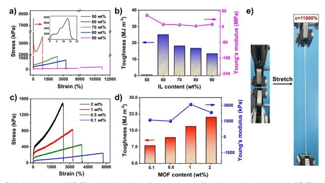
Fig. 2 Mechanical properties of UiO-66-ionogels. (a) Monotonic tensile stress-strain curves, (b) toughness, and Young's modulus of the UiO-66-ionogels with different IL contents and 1.0 wt% UiO-66. (c) Monotonic tensile stress-strain curves, (d) toughness, and Young's modulus of UiO-66-ionogels with different UiO-66 contents and 80 wt% IL. (e) Stretchability of the UiO-66-ionogel (IL: 90 wt%, UiO-66: 1.0 wt%) up to 11 000% of the original.
