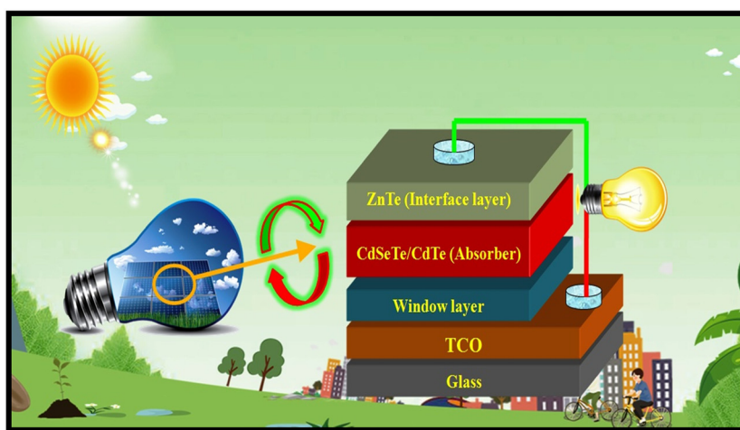
Fig. 13 Pictorial view of ZnTe back contact comprised of CdSeTe/CdTe thin film solar cell device structure together with natural conditions.
