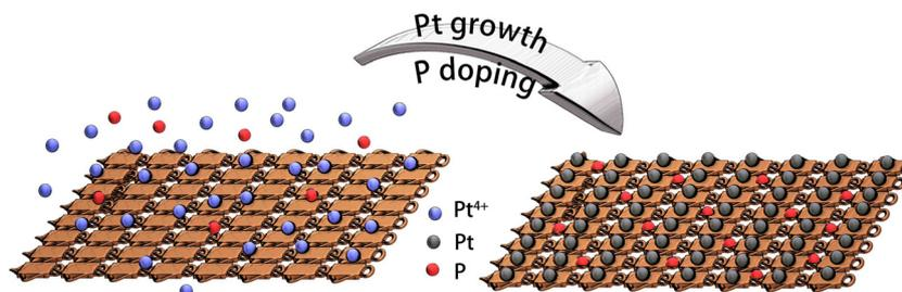
Fig. 1 Fabrication process of phosphorus-modified Pt@Cu (Pt/P@Cu).
