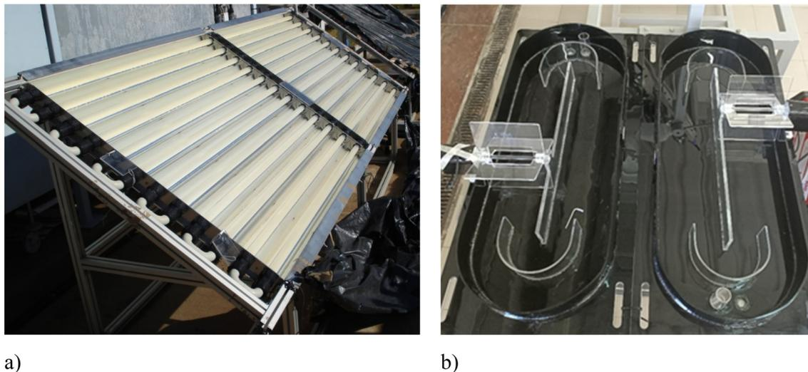
Fig. 3 CPC-based reactor (a) and RPR plant (b).
